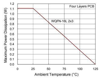
Figure 2. Derating Curve for RT9385B Package
